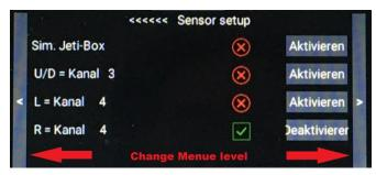
The buttons of the JetiBOX are controlled via 2 or 3 servo channels. Channel 3 is preset for the UP and DOWN buttons, and channel 4 for
