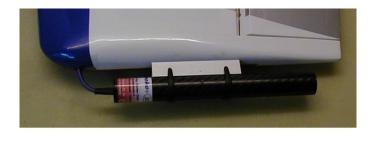
Please install the tubes for the RedOil and a two-core cable (2.5mm²) within the wings. The connectors for the tube and the cable are included in the set. Make sure you have the right polarity for each plug; the polarity is imprinted on the plugs.
