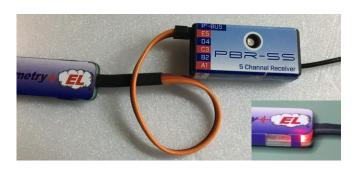
If the receiver is switched on, a red LED lights up in the Tele-Bridge.
