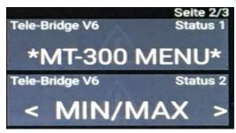
Usually, you can access the sensor menu by pressing the [DOWN] key. Activate the function that you have set for [DOWN]. In our case, channel 3 down. Make the desired settings.
