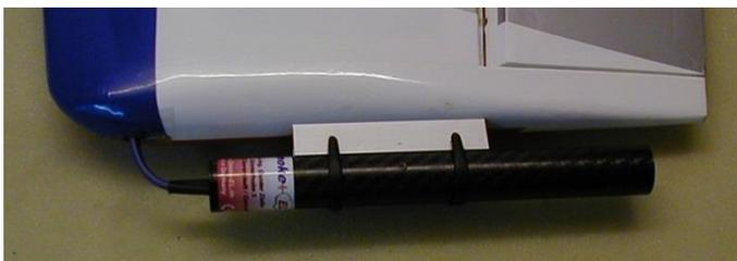
Please install the tubes for the RedOil and a two-core cable (2.5mm<sup>2</sup>) within the wings. The connectors for the tube and the cable are included in the set. Make sure you have the right polarity for each plug; the polarity is imprinted on the plugs.
