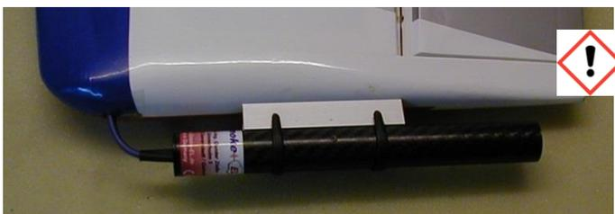
**Please note: the housing of the smoke-tube is connected with the negative pole and therefore not potential-free**
